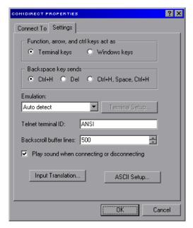
Figure 11: HyperTerminal Properties...Settings
